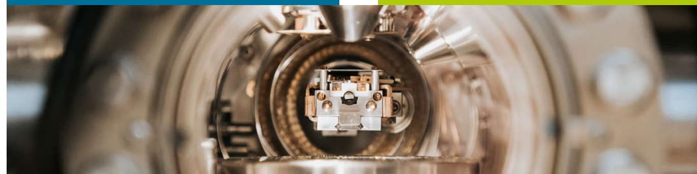
View into the sample chamber of the X-ray photoelectron spectrometer at LENA, the research centre for nanometrology. Photo: Markus Hörster/TU Braunschweig
