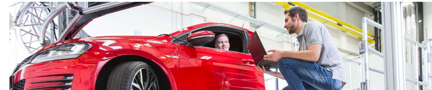
The full-vehicle simulator at the NFF automotive centre enables research not only on vehicle control systems, but also on new driver assistance features and self-driving functionalities. Photo: Christian Bierwagen/TU Braunschweig
